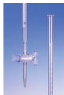
Straight stopcock with glass spindle
